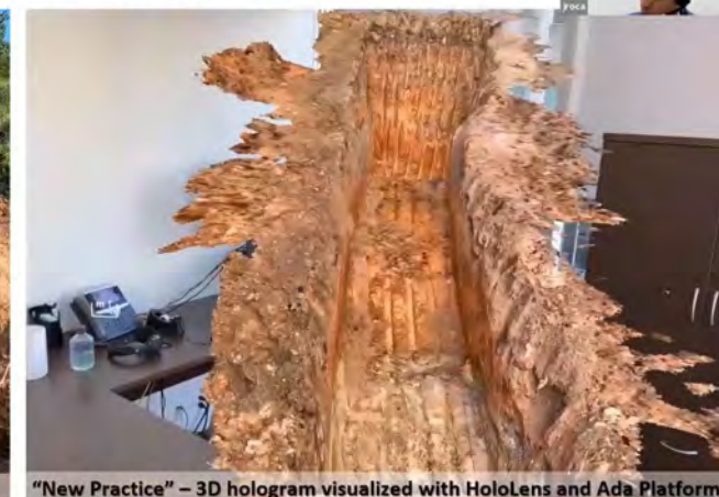
Collect Field Data – Test-Pit Example at Dam Foundation
