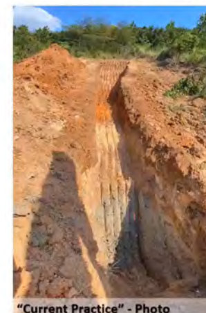
Collect Field Data – Test-Pit Example at Dam Foundation
